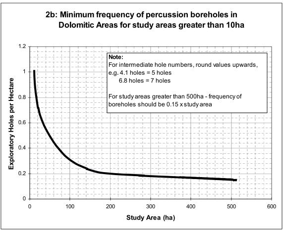
Figure 2: Minimum frequency of percussion boreholes in Dolomitic Areas
