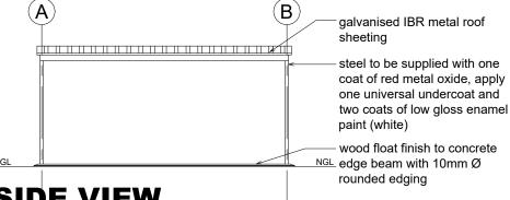
galvanised IBR metal roof sheeting steel to be supplied with one coat of red metal oxide, apply one universal undercoat and two coats of low gloss enamel paint (white) wood float finish to concrete NGL edge beam with 10mm Ø rounded edging
