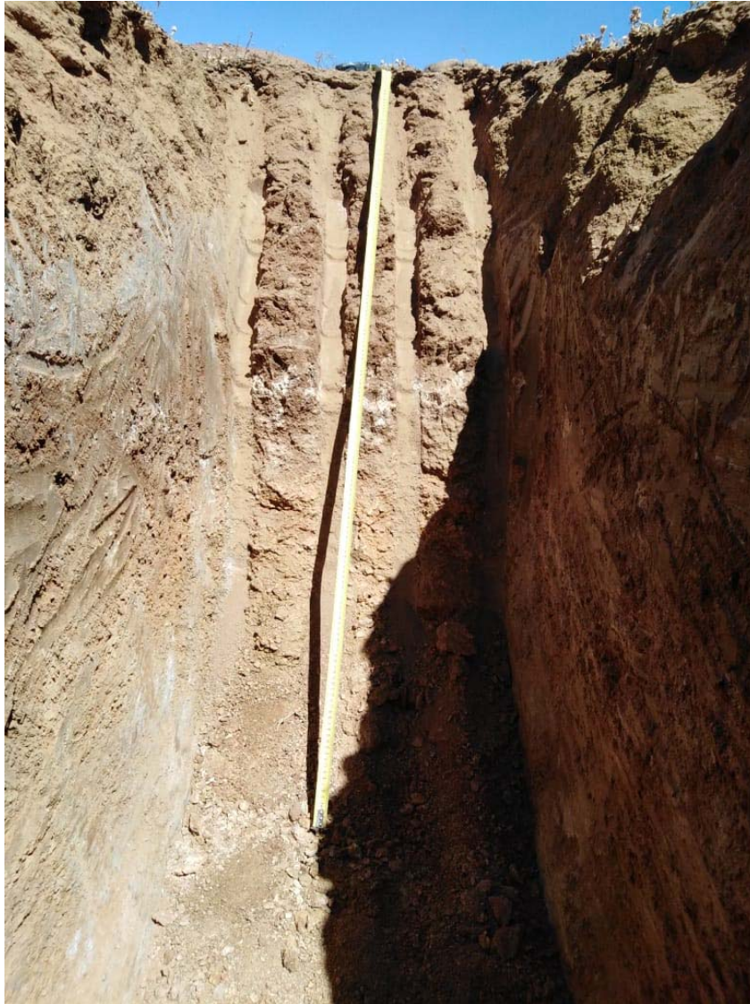
Figure 5: Showing a typical test with residual Granodiorite.
