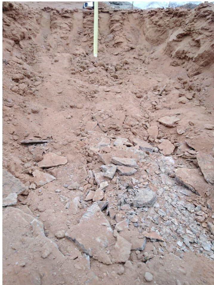
Figure 9: Showing a typical test pit where refusal was on gneiss bedrock.
