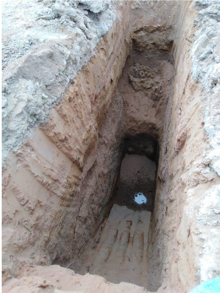
Figure 10: Showing water seepage in the test pit.
